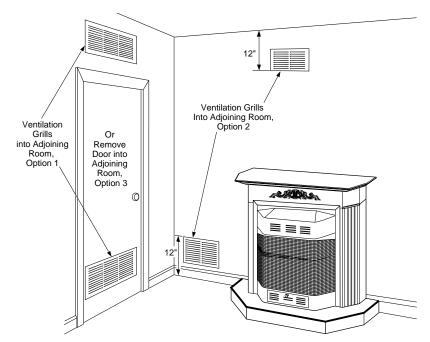
Figure 2 - Ventilation Air from Inside Building Shown with Optional Mantel
